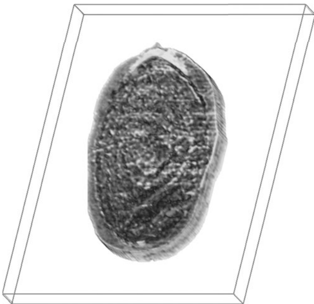
Fig. 8. Surface visualization of the AFM 3D reconstructed cyanobacteria Synechococcus , which was high-pressure frozen and epoxy freeze-substituted. The resulted volume image contains 432 \times 398 \times 6 voxels what corresponds to physical size of 2.7 \times 2.5 \times 0.15 \mu\text{m} . The ImagePro Plus 5.1 3D Constructor software was used for the automatic image alignment by the correlation-based algorithm.
