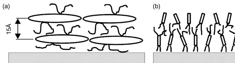
Fig. 7. Schematic picture of the orientation and of the molecules relative to the substrate surface is a side view (a) and in a front view (b).
