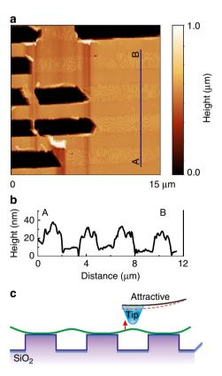
**Figure 1 | Topography of the sample. (a)** Measured in the tapping mode topography of SLG on the grating. Left part represents graphene damaged under scanning. **(b)** Cross-section along the line A-B showing supported and suspended graphene areas. Suspended graphene is about 20 nm higher than the supported one. **(c)** Schematic of the graphene and substrate arrangement explaining the origin of the observed bending.
