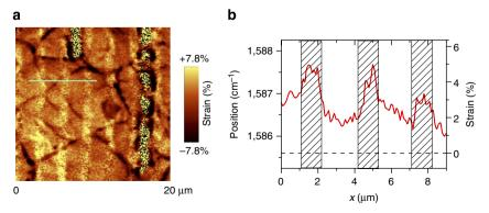
Figure 2 | Spatial distribution of strain over the sample structure. (a) Strain map of SLG on the Si/SiO<sub>2</sub> grating. (b) Variation of G-band position and strain across the grating (blue line in a); shaded rectangles correspond to supported graphene; dashed line denotes the initial (unstrained) value of G-band position.
