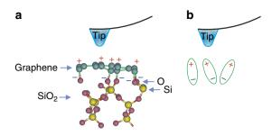
**Figure 6 | Origin of the measured piezoresponse.** (a) Schematic of graphene layer on SiO<sub>2</sub> substrate with oxygen termination. (b) Formation of Chemical interaction of carbon and oxygen atoms induces dipolar surface states oriented close to normal of the substrate surface.
