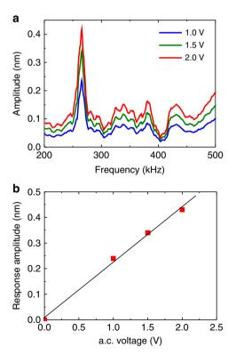
**Figure 5 | Piezoresponse measured versus a.c. frequency and voltage.**(a) Frequency dependence of PFM amplitude at different a.c. field levels near the first contact resonance measured on supported graphene layer.
